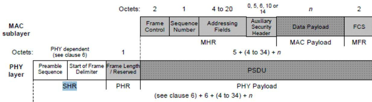
The last 2 bytes of PSDU are CRC bytes for the 802.15.4 FCS (Frame Check Sequence). The radio hardware computes and transmits these 2 bytes automatically, so software need not load them into the Packet Buffer. Thus, for TX sequences, the number of bytes to
